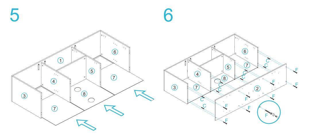
Slide panels [7] and panel [8] into position as shown.
