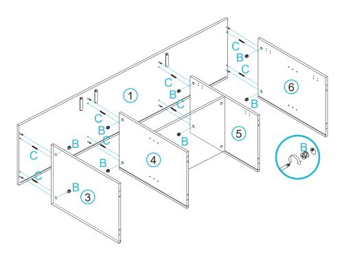
Attach panels [4] and [5] to panel [9] and secure with 4 x dowels (C) and 4 x nuts (B). Tighten with a screwdriver.
