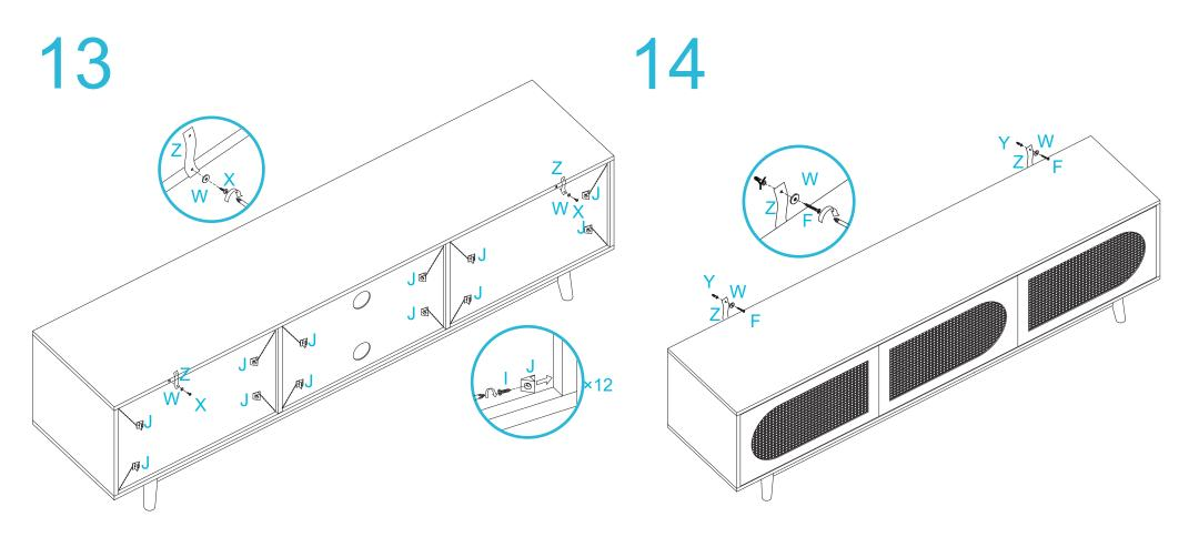
Attach 12 x wedges (J) as shown and secure with 12 x screws (I). Attach 2 x safety straps (Z) and secure with 2 x washers (W) and 2 x screws (X). Tighten with a screwdriver.
